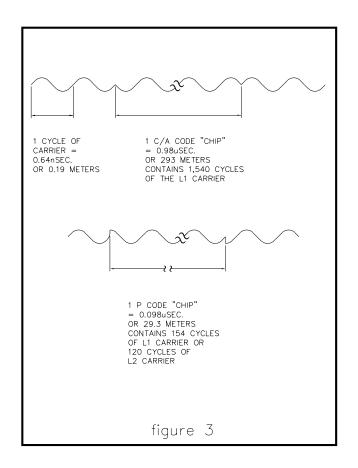
Data being sent on the carrier is represented by either inverting or not inverting the PRN code, so that at the receiver the correlator will generate either a positive or negative correlation output. The data rate is usually much slower than the chipping rate so that it does not interfere with the integration that is done as part of the correlation process. Data on the GPS signals, called the Navigation Message, are modulated at a nominal 50 bits per second rate.
