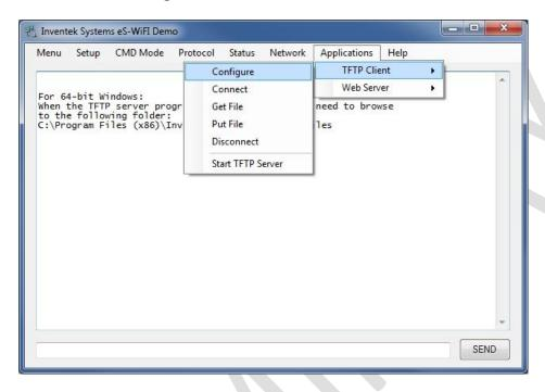
Now enter the IP Address of TFTP Server (from above it would 192.168.1.154). You only need to change the defaults when using different files. Once entered click the OK button.
