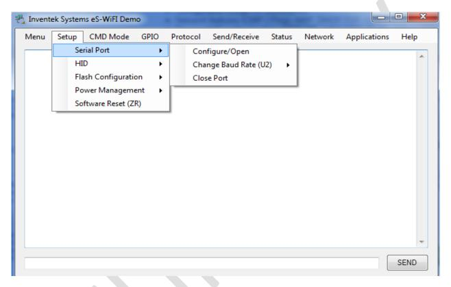
You will now configure the VSP (Virtual Serial Port) connection the EVB. You will need to determine what COM port is attached to the EVB. This can be done by using Windows Device Manager. In this case, COM54 is the port connected to the EVB.
