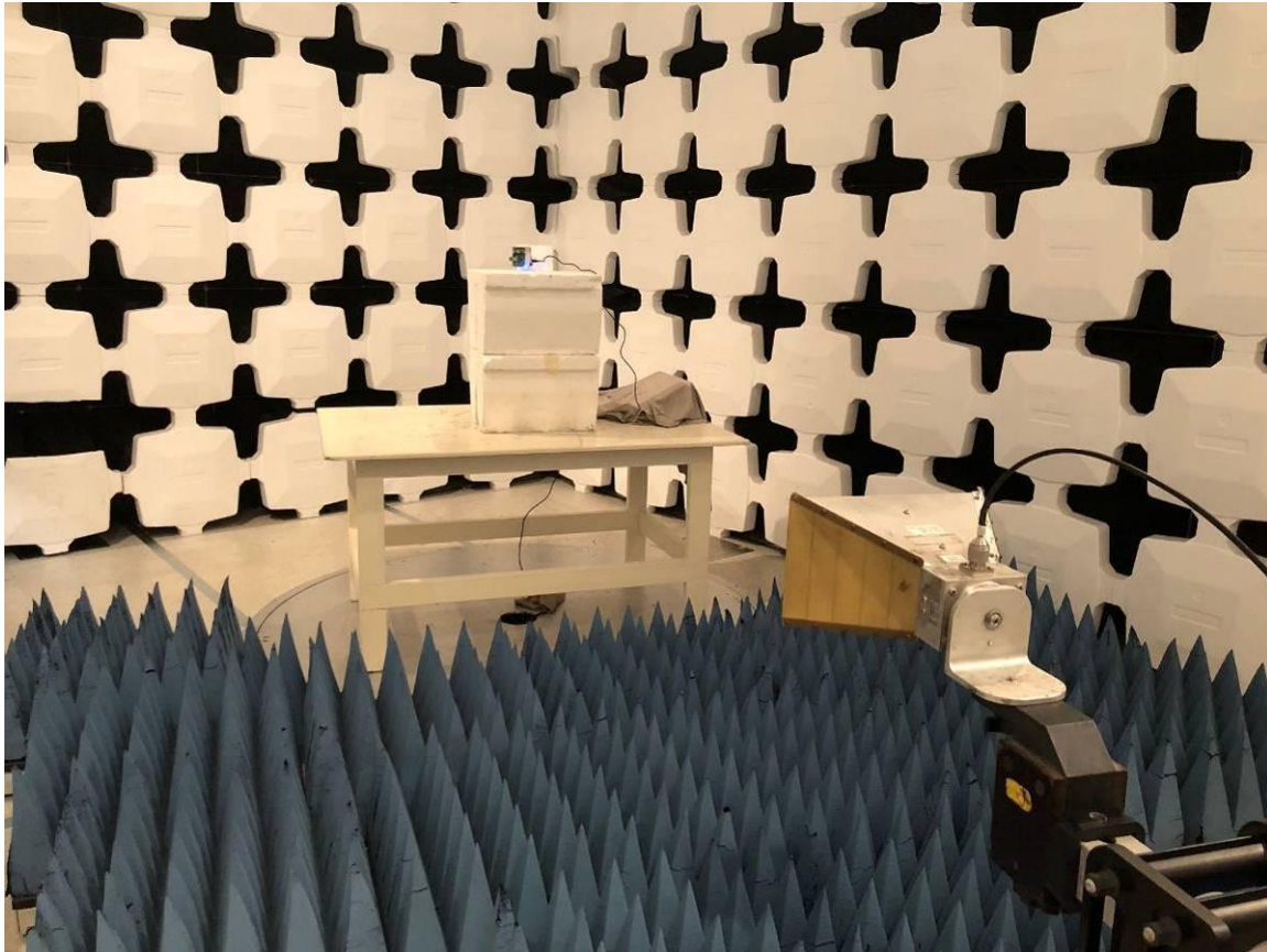
Figure 67. Radiated Spurious Emissions Above 1000 MHz
