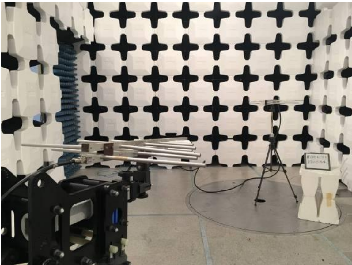
Figure 69. 200-1000 MHz Substitution Testing
