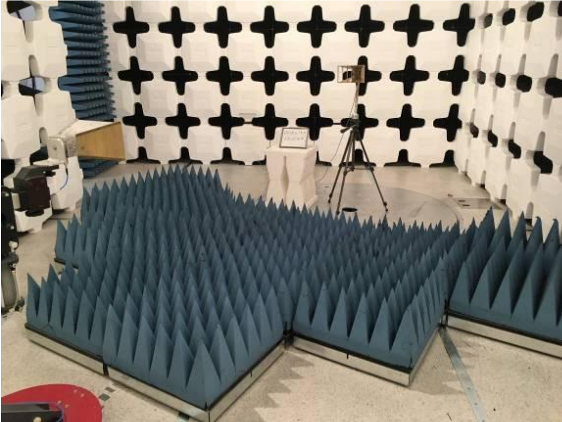
Figure 70. Above 1 GHz Substitution Testing
