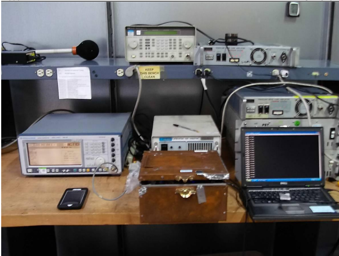
Figure 73. Receiver Blocking Test Setup
