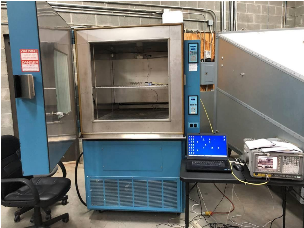
Figure 71. Extreme Temperature Test Setup
