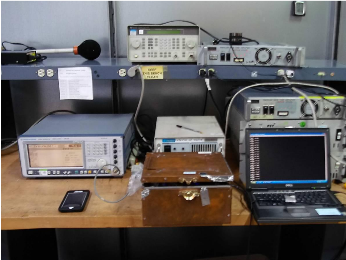
Figure 38. Receiver Blocking Test Setup
