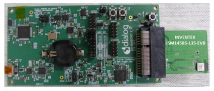
The ISM14585-L35-EVB Daughter Card Evaluation Board is a pin to pin compatible evaluation board that seamlessly interfaces to the Dialog DA14585 Development Kit-Pro Mother Board including application support via Dialog's SDK -SmartSnippets Studio and downloaded via USB (USB to UART transfer IC) to the ISM14585-L35-EVB.
