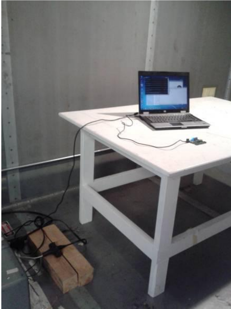
Figure 19. Conducted Powerline Emissions Test Setup
